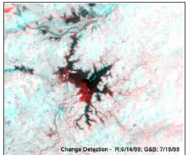
Fig. 5 Change detection using two AVHRR images (June, July, July in R,G,B respectively): the flood extent on July 19<sup>th</sup> appears in red.
