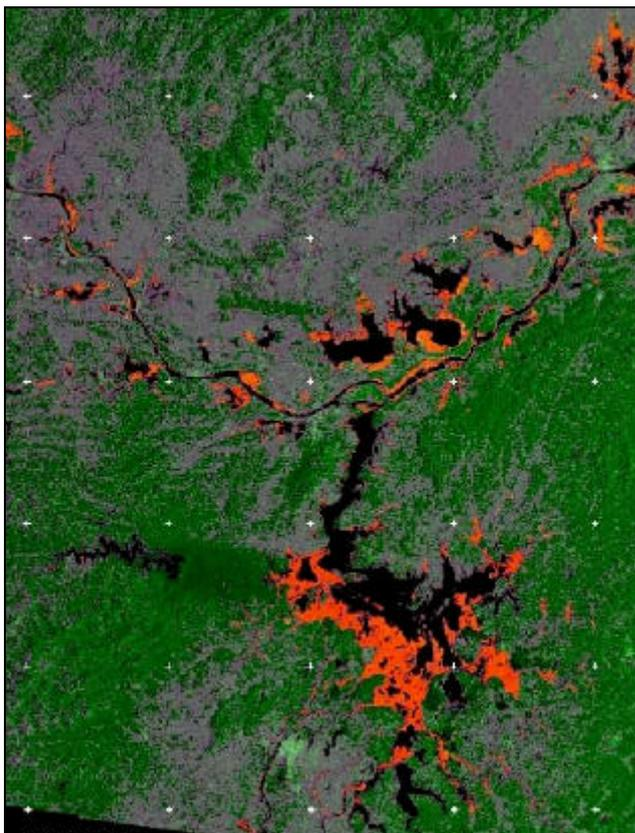
Fig. 4 A HSV visualisation using the change detection between the archive and the July acquisition, with the archive image as a background. Interpretation: flooded areas in orange; saturation with water in grey
