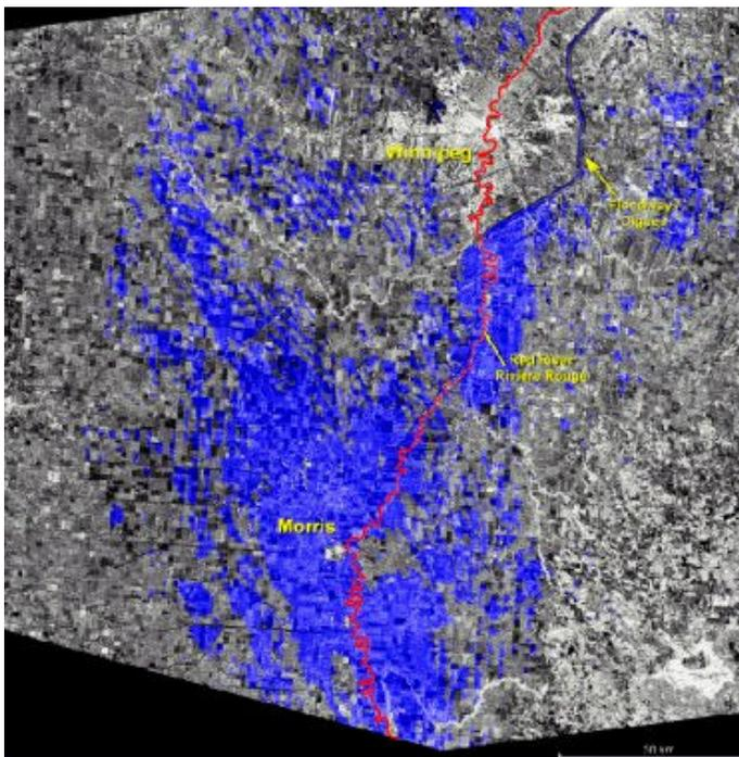
Fig. 7 A RADARSAT Standard 2 Desc. (April 27, 1997) captured the extent of the Red River flood (Canada/US border). The flooded region is colored in blue for ease of interpretation.
