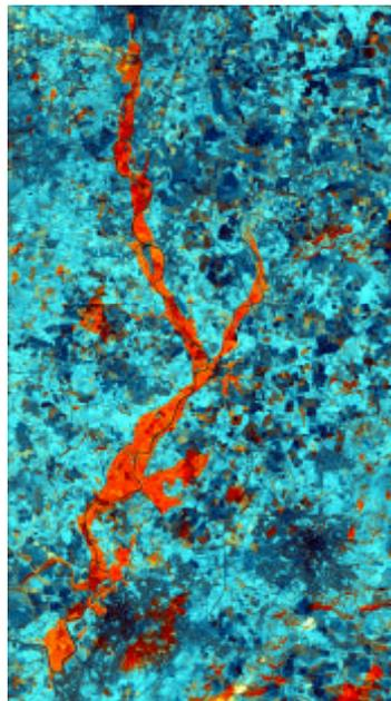
Fig.1. The flood map resulting of the HSV composition and of the change detection between SPOT 4 and SPOT 1 (using the latter image as a background) shows the flood extent on November 1<sup>st</sup>
