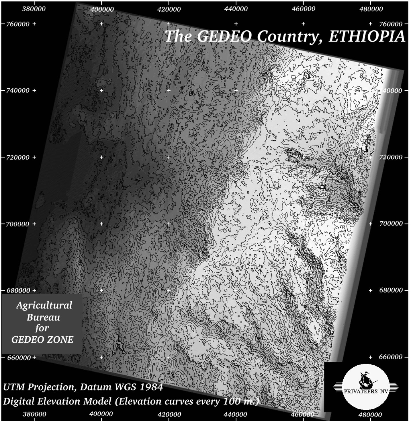
Figure 3: The Digital Elevation Model (DEM) of Gedeo Zone (Ethiopia), in Universal Transverse Mercator (UTM) cartographic projection, with superimposed elevation curves.
